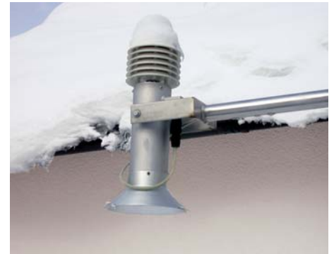
Fig. 9: Ultrasonic snow gauge type USH-8 (Sommer Ltd.) in action at Siedlinghausen
